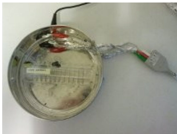
Figure 3.11 The Faraday Cage, the Nerve Chamber and the Bio Amp Cable
