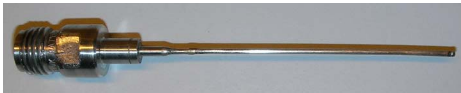
Figure 3.4: The pressure cell used in pressure experiments. To the right is the capillary which holds the sample. To the left is the head which is attached to pressurized nitrogen.
