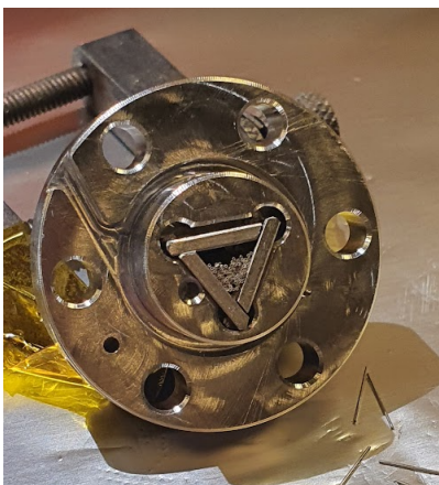
Figure 3.17: Filling the oven lid with micro capillary tubes. The triangular arrangement of steel plates can be tightened to push the tubes into a stable honey comb structure.
