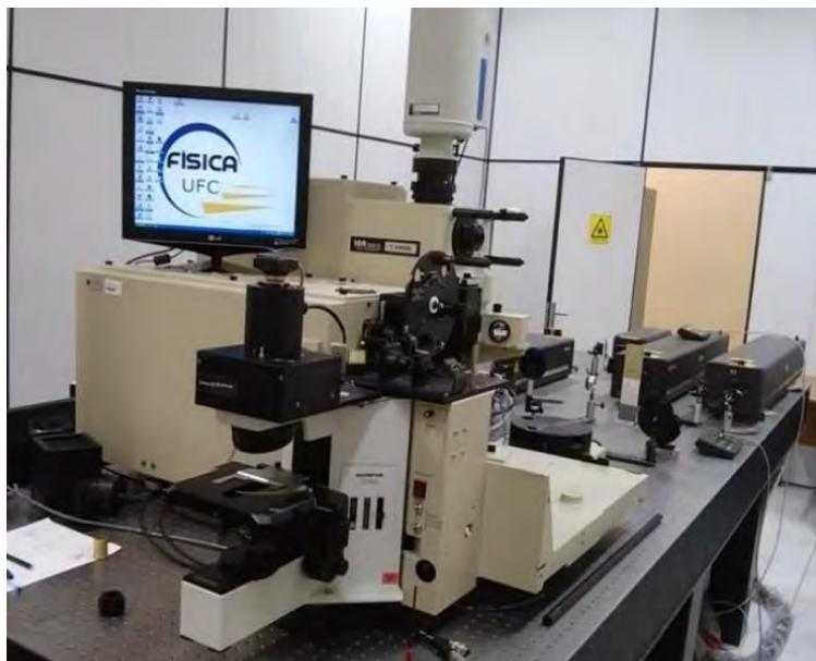
**Figure 13** Picture of the Horiba T64000 triple spectrometer used for polarized Raman measurements located at Universidade Federal do Ceará (Brazil).
