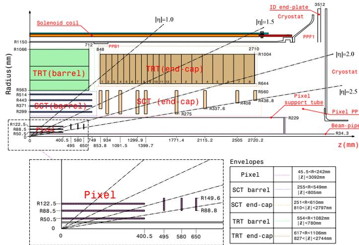
**Figure 3.9:** Scheme of the ATLAS inner detector with the description of the barrel and the end-cap regions of each inner detector subpart.
