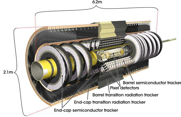
**Figure 3.8:** A view of the ATLAS inner detector.
