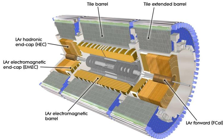
Figure 3.10: A schematic view of the ATLAS calorimeter.
