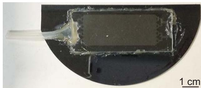
**Figure 6.12:** Simple SU-8 microfluidic channel (type A) on a half 4 inch substrate plasma bonded to a PDMS coated glass slide (type X). The seal has been tightened and one inlet glued on with epoxy.
