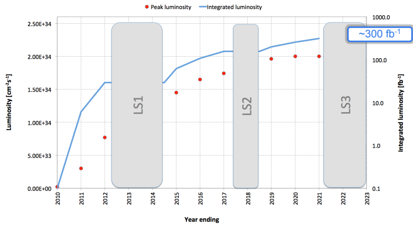
Figure 10.1: Planned baseline evolution for the LHC. We were in the LS1 period when this was written in the winter of 2014. Ref. [25].
