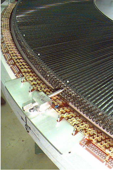
Figure 6.9: A layer of the TRT end-cap being assembled http://www.hep.upenn.edu/atlas/trt/ .
