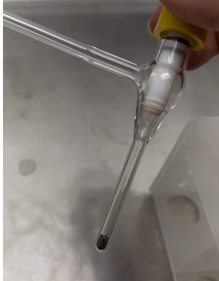
Figure 7.1: Iodine in our experiment is transported under a fume hood into a Young valve.
