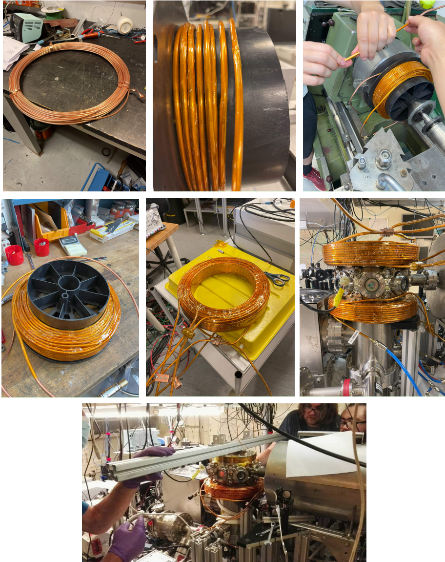
Figure 3.1: Winding of the hollow tubing MOT coils. Top row shows how it looked when it was newly purchased and us winding it on a lathe, coating it in kapton tape as we went along. The second row is a finished coil, which we then tested the water cooling and magnetic field before removing the vacuum chamber and placing it on the experiment in the bottom picture.
