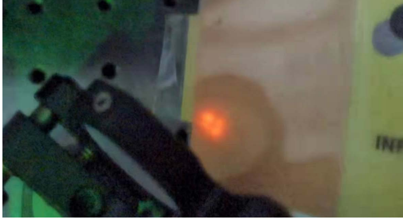
Figure 43: The mode shape can remain as the beam shape after leaving the cavity for about 200mm. Here the beam waist on the membrane is 2w_0 = 37\mu\text{m} .
