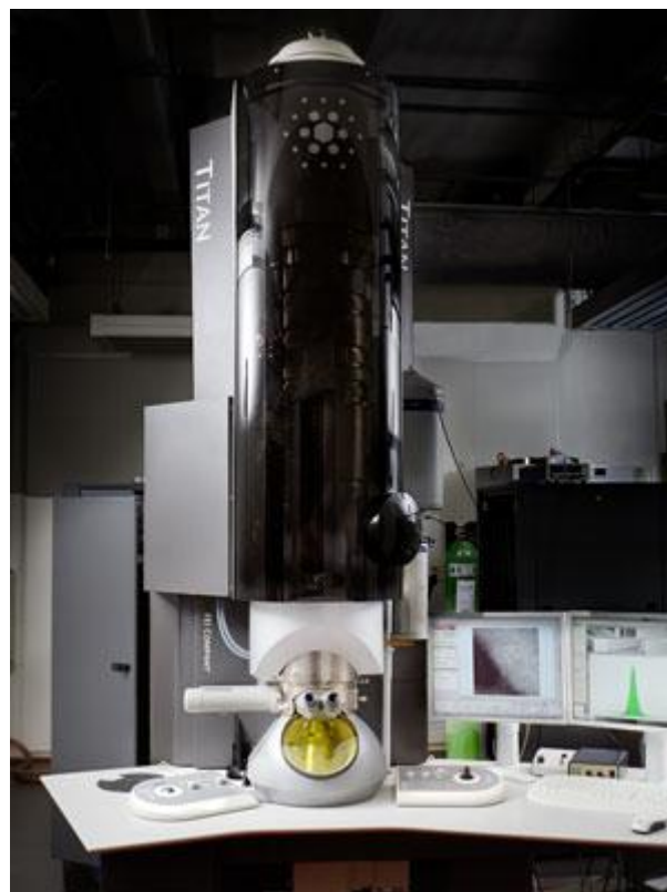
Figure 3.4: The photo of FEI TITAN microscope
