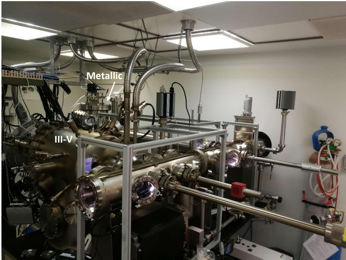
Figure 3.1: The photo of the MBE system for sample preparation. The III-V growth chamber is marked with “III-V” and the metallic chamber is marked with “Metallic”.
