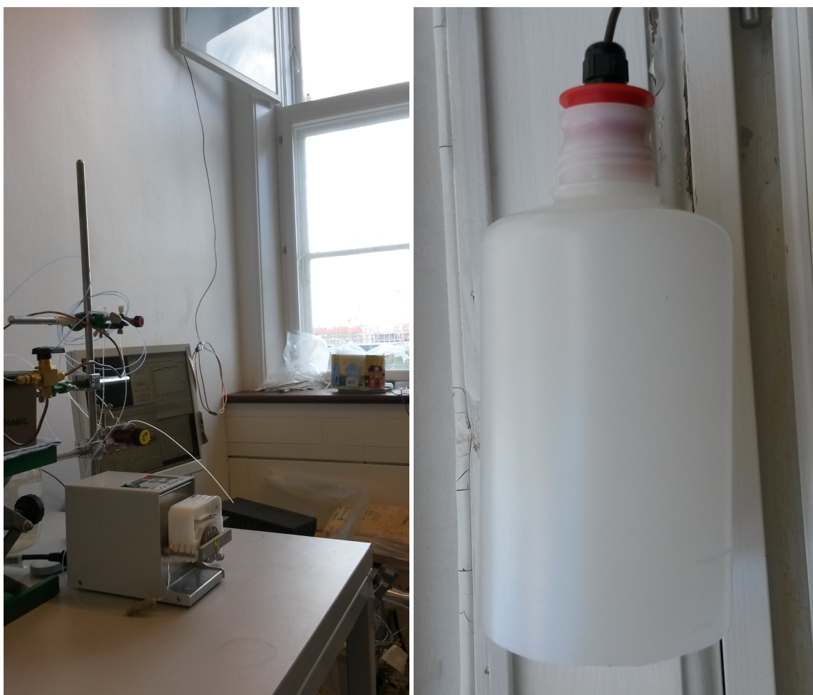
Figure 3.4: Left image: the copper tube of the vapor line that exits out of the room to collect atmospheric vapor. Right image: the plastic bottle for sampling atmospheric water vapor. Its top is sealed with expandable polystyrene in order to ensure that we are only sampling vapor and no precipitation is entering to the vapor sampling line through the plastic bottle.
