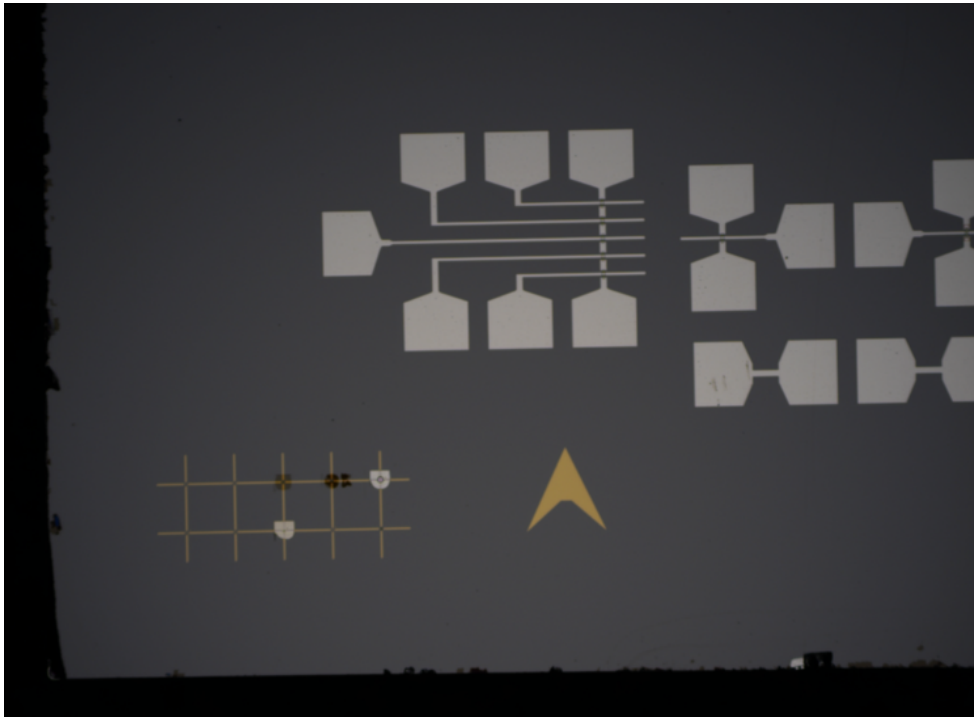
Figure 3.5: Optical image taken in the lower left corner of the finalized crossover chip. The grey is the InP substrate, the white is the control layer aluminium, the gold is alignment marks and an orientation arrow; made of gold.
