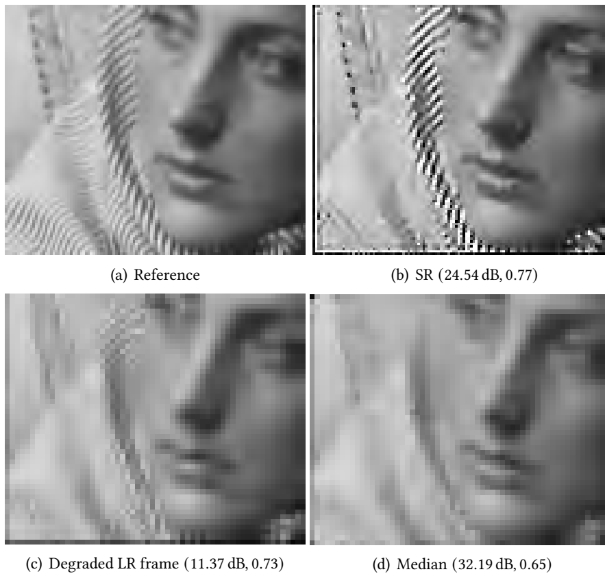
Figure 3.11: MFSR image of Barbara. Magnified by a factor of s = 2 in steps of \Delta s = 0.1 , from a size of 60 \times 50 to 120 \times 100 . The LR frames were created by random subpixel translations in the range of 5 pixels, blurred by a Gaussian blur of \sigma = 0.5 and downsampled to half the original size by nearest-neighbour interpolation. The regularization parameter \lambda = 0.0008 was found through cross-validation and the total runtime was 212 s. The median and one of the degraded LR frames upsampled by bicubic interpolation to that of the original image. The first measure is the PSNR and the second measure is the SSIM.
