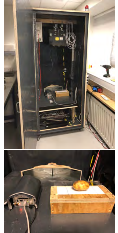
Figure 4.10: X-ray imaging system located at NewTec (top) full view (bottom) close-up. The setup consisting of an X-ray generator, object of interest (potato) lying on a scintillator sheet and a camera. Image from the master thesis by Aleksandar Topic
