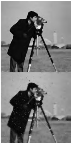
Figure 2.28: (top) noise removal by median filter of size N = 5 . (bottom) bilateral filter of size N = 9, \sigma_s = \sigma_r = 100 .
