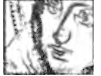
Figure 3.10: Example of the \alpha map, represented by the sum of the gradients found in all directions for the temporal median of the degraded Barbara sequence
