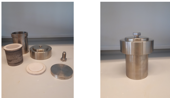
Figure 28: Picture of a disassembled stainless steel hydrothermal vessel and an assembled one, respectively. This vessel can contain 80 mL, and is custom made by the workshop of Department of Physics, Chemistry and Pharmacy at University of Southern Denmark.
