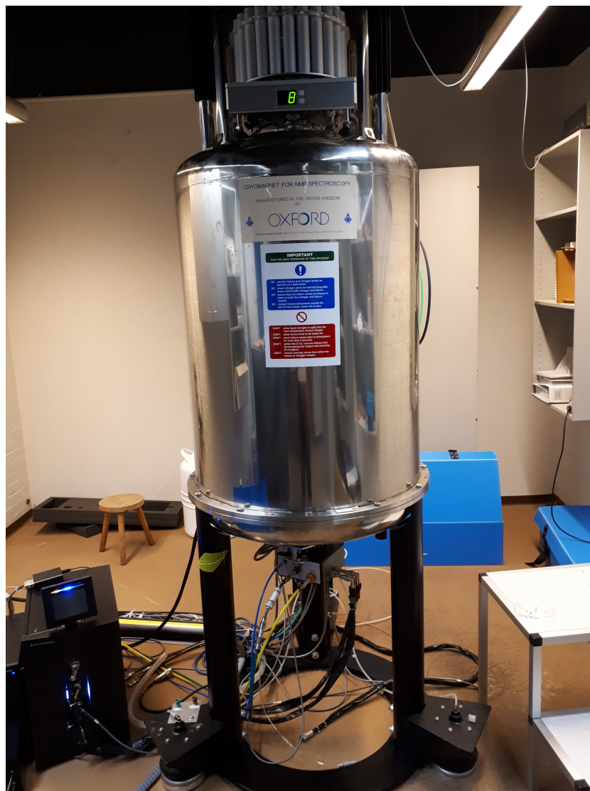
Figure 17: The JEOL 500 MHz NMR spectrometer with a 11.7 T Oxford Magnet at SDU, which has served as the primary NMR instrument for this study.
