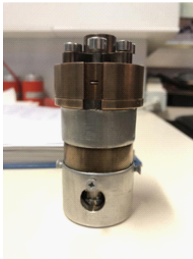
Figure 6.1: Image of the pressure cell v2. The cell has been covered in a sheet of cadmium, everywhere but at the sample position.
