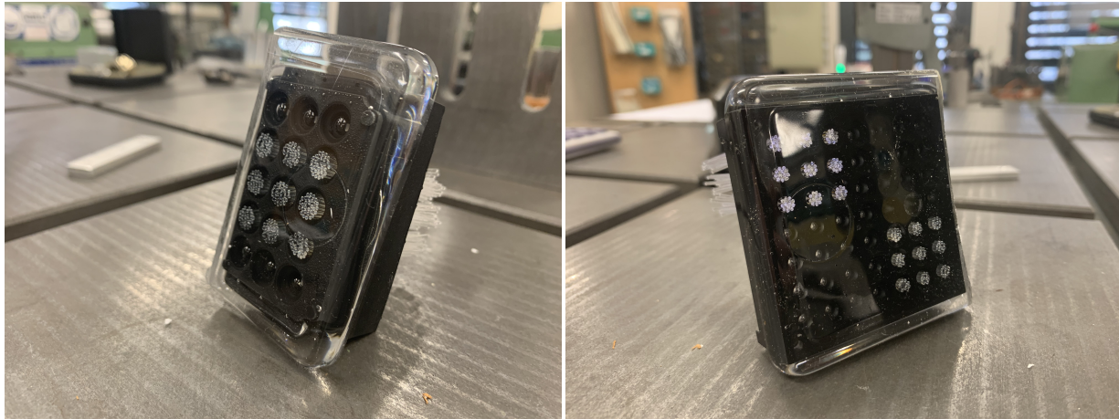
Figure 35: The two pictures show two collector plates of two different materials, after the fibers have been glued with optical glue. The left-side figure shows the collector plate made of the material called resin. The right-side figure shows the collector plate made of 3D filament.
