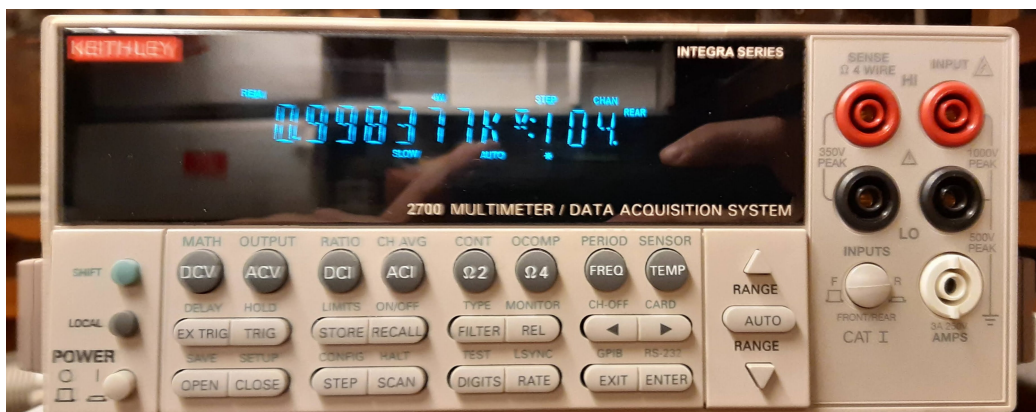
Figure 5.10: The Keithley 2700 Digital Multimeter is used to probe a set of 9 thermocouples placed throughout the superconducting magnet and pulse tube compressor, the data allows us to keep track of the cooling process. It is connected to the cryogenics station using a serial port.
