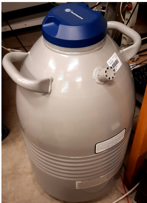
(a) An image showing the dewar that holds the liquid nitrogen used to cool the trap.
