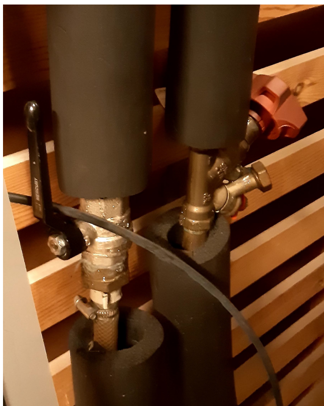
Figure 5.22: An image showing the valve controlling waterflow to the turbopump, it is open in this case. When the turbopump is running it needs watercooling, but when the setup is idle we can turn off the waterflow to minimize the likelihood of contamination or a leak.
