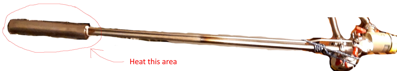
Figure 5.21: An image showing the trap in full size (though rotated), encircled is the area containing the activated charcoal, which can be cleaned of impurities by heating with a heat gun.
