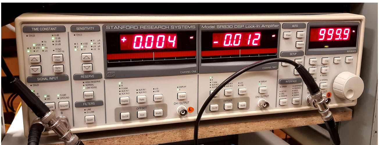
Figure 5.5: The Stanford Research Systems SR830 DSP Lock-in amplifier is used to measure the complex (ac) voltage induced in the measurement coils, it is controlled through a GPIB interface to the magnetism station.
