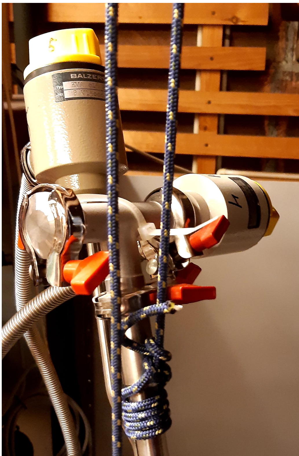
Figure 5.16: An image showing the manual valves that control flow through the trap, which filters impurities out of the helium mix. These need to be turned to open, and must be opened for helium mix to flow through the system.
