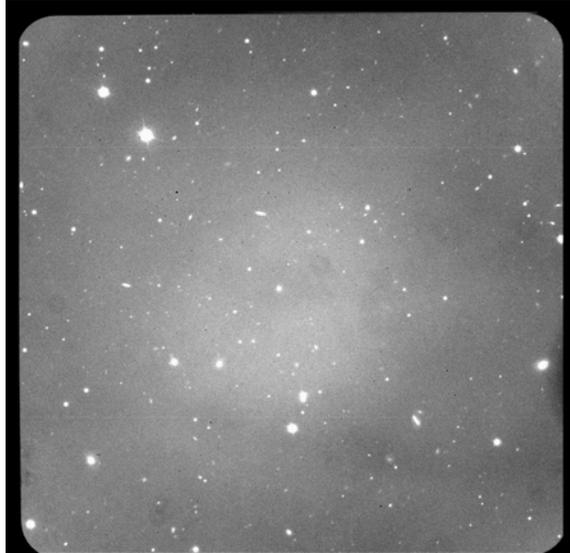
FIGURE 7: An unprocessed science frame. The overscan is visible towards the edges. The brighter glow towards the center is not an actual astrophysical signal, but it is the effect of pixel-to-pixel response variations that will be corrected for in the flat fielding.
