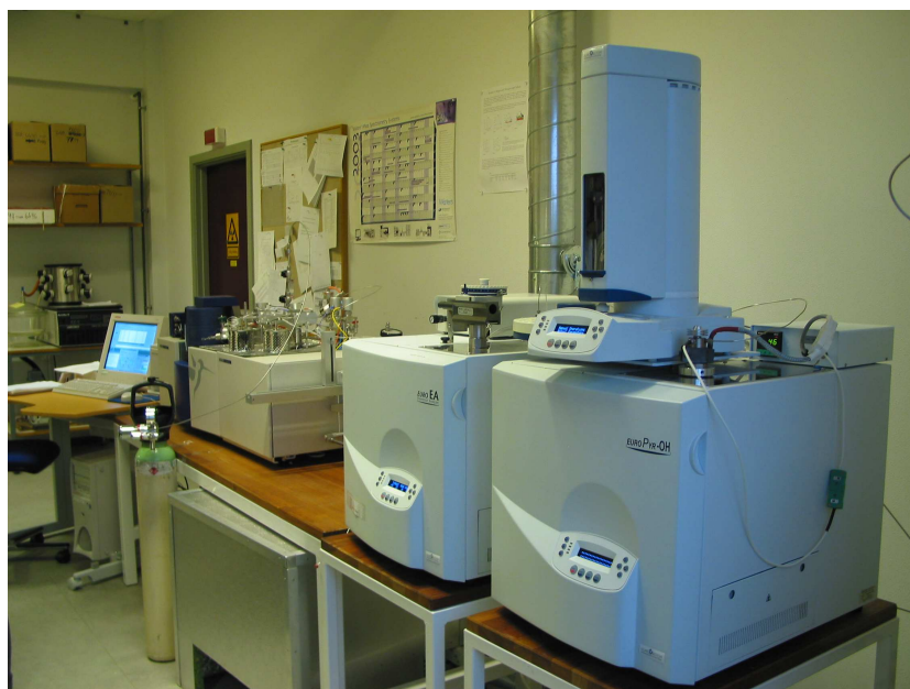
Figure 5.1: Experimental set-up. From right to left: Liquid auto sampler, elemental analyser, Isoprime mass spectrometer and computer. See Figure 5.2 for a schematic illustration.
