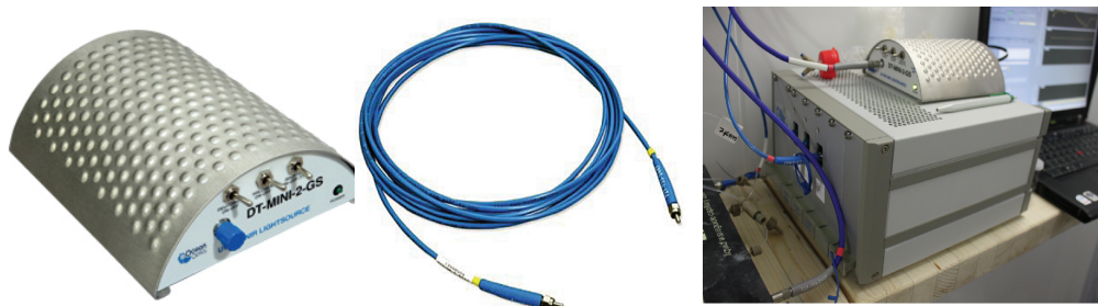
Figure 77: The lamp, optic fibres, and spectrometer used in the set-up.
