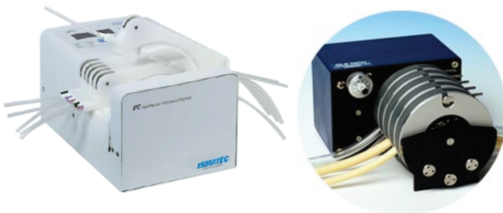
Figure 78: The two types of pumps used for the measurements. Left, ISMATEC. Right, Ole Dich.
