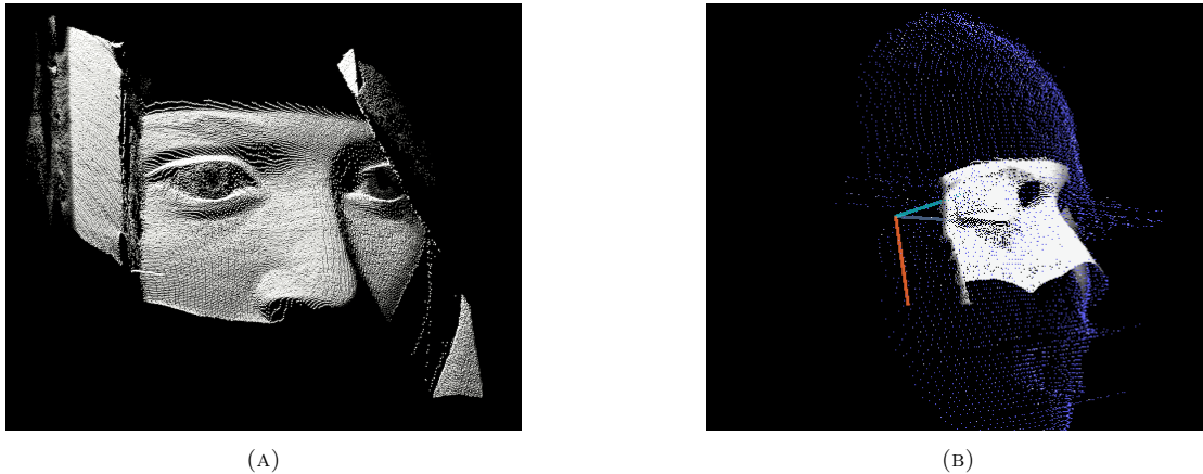
FIGURE 13: (A) Point cloud example visualising the camera field of view of a subject within the head coil. (B) Cross calibration between face selective MR scan (blue) and Tracoline point cloud (white).
