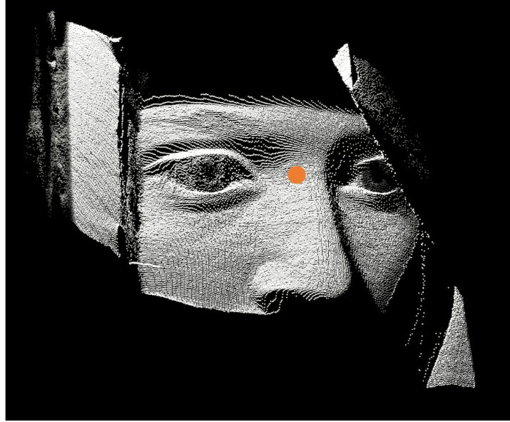
Figure S.3: Example of the Tracoline point cloud for an adult. The point cloud centroid is schematically visualised by the orange circle. Please note that the field of view varies with head size and curvature of the face; for children a larger part of the face might be covered.
