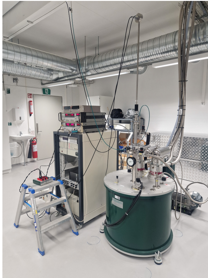
Figure 6.31: 16 Tesla Cryostat setup
