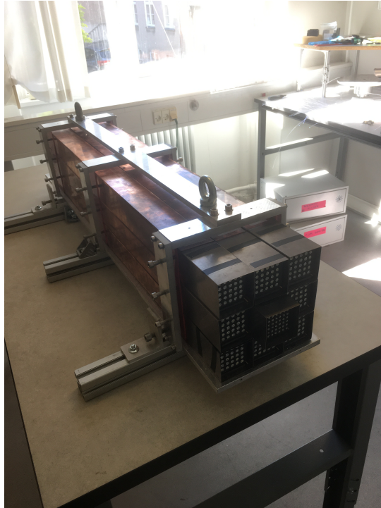
(b) The full prototype as viewed from the back, giving a view of all the bundled straws.
