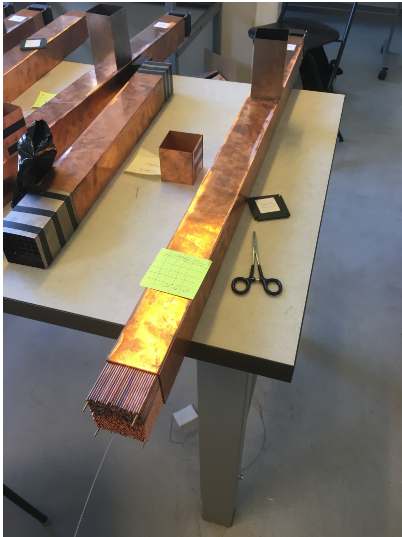
Figure 15: One of the 9 modules of the second prototype during the process of inserting the fiber straws
