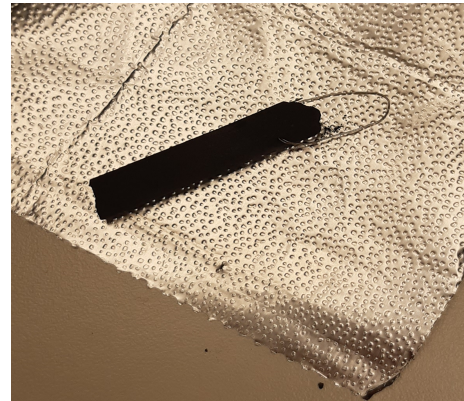
c) 40mm pressed rod with platinum wire.
