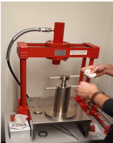
b) Retrieving sample from hydrostatic press
