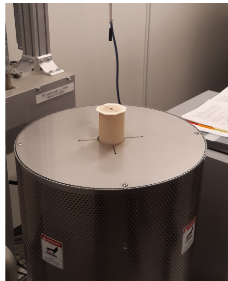
d) Sintering rod in vertical furnace
