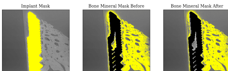
Figure 6.9: Improving on the bone mineral segmentation by limiting the bone mineral segmentation to outside the implant. The segmented implant mask for slice n = 60 (left), the original segmented bone mineral mask (centre), and the improved segmented bone mineral mask (right).
