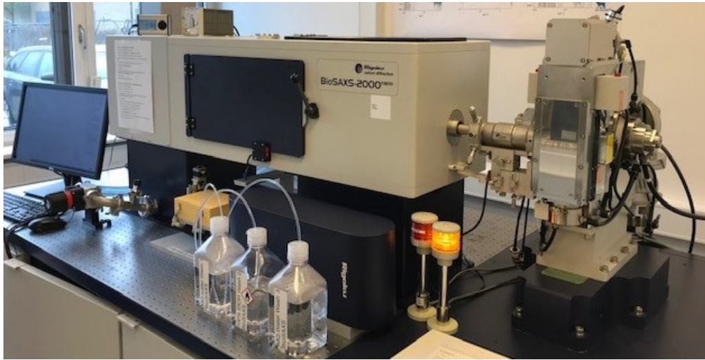
Figure 7.2: Photo of the BioSAXS-2000 used for all SAXS and WAXS experiments of this work.
