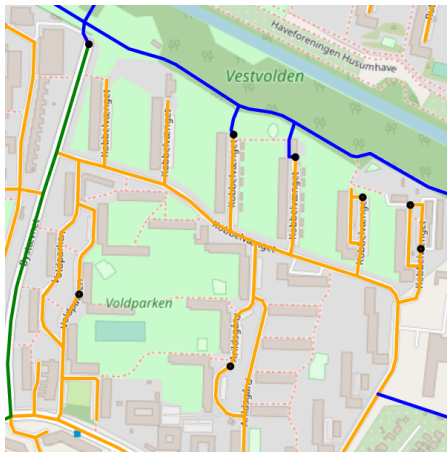
Figure 2.7: Preserved nodes of degree 2 in the simplified network. Car links are shown in orange, multi links in green and bicycle links in blue. Only nodes of degree 2 (black circles) are shown. All preserved nodes of degree 2 are either meeting points of links of two different types (as the three nodes in the upper left part of the figure) or belong to a loop (remaining nodes). [107]
