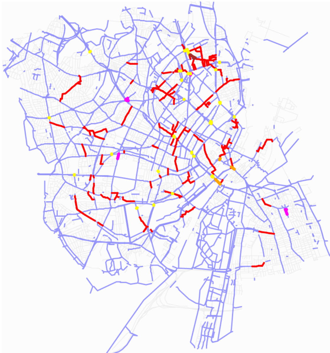
Figure 3.7: Overview map of top 101 gaps by class: missing links in red, bridges in orange, intersections in yellow, right-turn lanes in pink, roundabouts in brown. Data issues are not shown. The street network is shown in grey, the bicycle network in blue.
