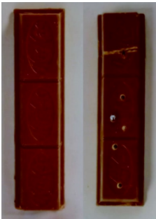
Figure 5.11: Selected RGB images of chocolate bars used for the case study. Left: normal sample. Right: added foreign objects and a vertical crack.
