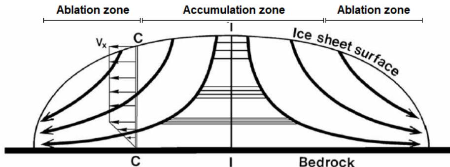
Figure 2: Idealised illustration of the ice flow, indicated by the thick arrows, through the cross section of a large glacier. The horizontal line around the ice divide,  $I$ , represent annual layers, which get stretched and thinned with depth.  $C$  marks an arbitrary position on the ice sheet and  $V_x$  is the horizontal velocity trough the ice cap. Taken from Bizet, B. J. R. (2006) [6].
