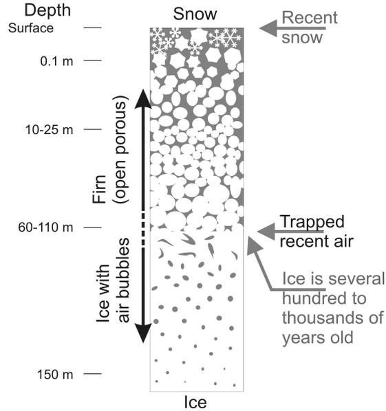
Figure 3: Schematic illustration of the transformation of snow to ice in an ice sheet on a depth scale. The different stages of transformation are indicated. Taken from *The firn zone: Transforming snow to ice* [7].
