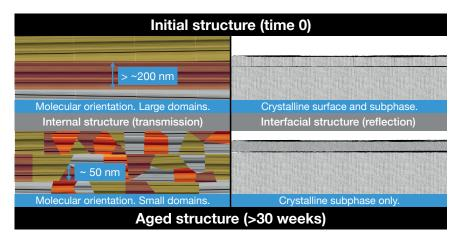
SAXS and XRD in combination show how the LCP structure changes with prolonged exposure to water. Initially, the LCP domains are larger than 200 nm but break down into smaller nanoscale domains after prolonged exposure. The material retains a high crystallinity and high degree of molecular orientation even when the domain size becomes small, but the crystallinity of the surface layer is lost after very long exposure times.
