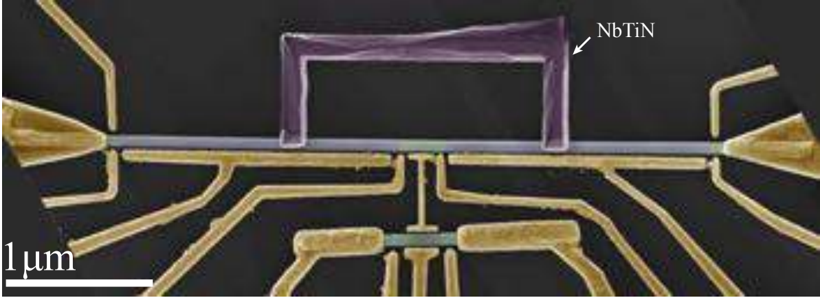
Figure 5.2: Loop Qubit devices. Double SC QD device with sputtered NbTiN loop that is connected to epitaxial Al of the nanowire. The device has a charge sensor nearby to read out the charge state of Majorana based qubit.
