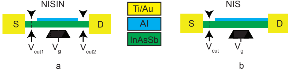
Figure 5: a) Schematic representation of the Copenhagen geometry (NISIN) device. The cutter gates, V_{cut1,2} , are used to tune the coupling to the source (S) and drain (D) contacts, while the plunger gate, V_g , is used to tune the chemical potential in the NW. b) Schematic representation of the Delft geometry (NIS) device. The cutter gate, V_{cut} , is used to tune the coupling to the source (S) contact while the plunger gate, V_g , is used to tune the chemical potential in the NW. Figure slightly redone from [55].
