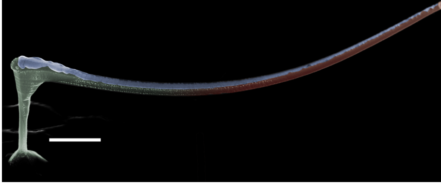
Figure 10: False-colored 45°-tilt SEM image of a Qdev253 WZ NW on the growth substrate. The Sb concentration in the NW gradually increases until it reaches its final concentration of \text{InAs}_{0.65}\text{Sb}_{0.35} as illustrated by the green to red transition. Scale bar is 500 nm. Image credit Thomas Kanne.
