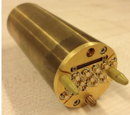
Figure 3.1: The puck used to load the sample. The yellow pins are guide sticks and the round connectors connect to the coax lines. The one used in this thesis is modified from this one. The large bus visible above the pins is sealed off, and the pins are female connectors.
